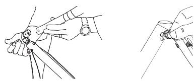
Do not insert the fitting at an angle, and do not force the fitting into the basetube if it does not slide in freely. Check for dirt or damage to the fitting or the inside of the basetube. If the fitting is forced into the basetube, it may be impossible to remove. See your dealer if the fitting becomes difficult to install or remove.
