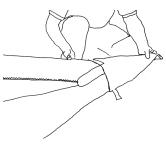
12. Install the plug-on #1 battens by inserting one end through the hole in the bottom surface at the tip and engaging the forked batten tip on the clevis pin standoff on the back side of the leading edge. Secure with a double loop of the 505 batten string.
