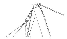
Check the condition of the sweep wires in the vicinity of the kingpost base bracket.
