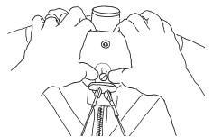
After installing the keyhole tang, rotate the aluminum anchor lock as shown to secure the tang on the bolt.
