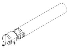
Shims are added to the allen screw type plug by sliding them over the end of the plug before the plug is inserted into the leading edge. The shims are thus visible with the plug installed.
