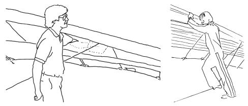
Open the crossbar junction access zipper and look inside, making sure that the safety ring on the junction bolt is in place and that the wires are secure and properly routed. Re-close the zipper.
