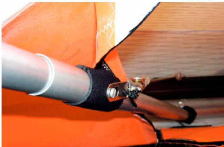
2.2.5. Look into the sail at each wing tip. Tip battens must be rested on the batten stop. The washout tip must be installed. Check for any evidence of dents, deep scratches, cracks or bends in the LE tubes. Be sure that the sail mount webbing is safely and correctly secured in the end cap slot (Fig. 10).
