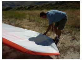
5. FIG. 5: Find the cross tube tensioning wire up inside the keel pocket. Then using the black webbing handle pull the cable back to snap into the spring catch. Now you will need to hook up the back top wire into rear spring fitting also.
