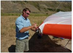
9. FIG. 7: Install the glider's nose shroud, starting with the two top velcro tabs and gently pulling the shroud down and around the nose plate to connect the two bottom velcro tabs on the shroud to its corresponding tabs sewn on the under-surface.
