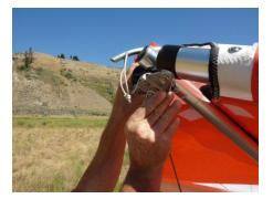
8. Install if necessary the nose batten "tail end first" from the nose of the glider seating the front end of the rib on the keel tube just in front of the nose plate.
