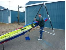
3. FIG. 3: Remove the cover and all the ties. Carefully walk each wing out to its approximate flying position. AT THIS STAGE IT IS ESSENTIAL TO ENSURE THAT THE KEEL AND LEADING EDGES ARE ALWAYS IN THE SAME PLANE.
