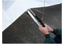
6. Install the tip batten. Look through the leading edge pocket at the wing tip and guide the tip batten onto the tip hook about 20" up the leading edge. Secure it with the same "double purchase" method described above in step 4.
