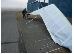
4. FIG. 4: Check the battens against the template and for symmetry. Placing all white rib fittings in the right wing, insert the battens from root to tip with gentle pressure, until the batten meets resistance, then lift sail at trailing edge and gently shake it in order to billow out. This enables the rib to be completely pushed into place over the cross spar.
