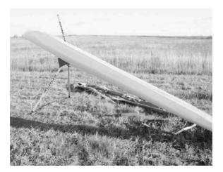
6. Spread the wings almost all the way. The kingpost will automatically rise half way up.
