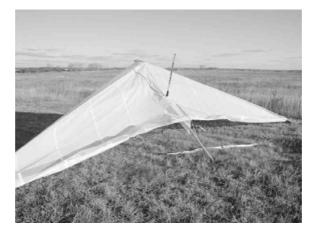
When spreading the wings make sure the washout bridles are not twisted or tangled around the bridle carabiner.
