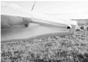
11. The next step is to install the outboard sprogs. To do so swing the sprog away from the leading edge and push it towards the leading edge in to the receptade. Make sure the sprog sits all the way in the sprog receptacle.
