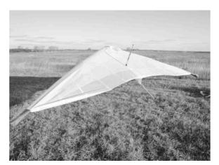
10. Install the last three cambered outboard top surface battens. Install the tip lever battens as shown on the photos.
