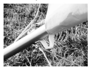
Check the nut of the kingpost channel, which secures the channel to the keel. Check the safety ring and the clevis pin, which secures the kingpost to the channel.
