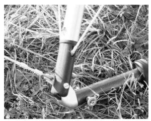
Check the sweep wire for wear where it passes through the kingpost channel.
