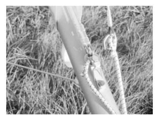
9. Pull the top rear wire backwards, the king post will stand all the way up. Attach the ring of the rear wire to the same hook on the keel tube on top of the sweep wire ring.
