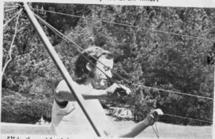
18. Slide the cable tighteners (nylon) to the black marks on the top rigging, and just snug on the tail wires (bottom). Overtightening can distort the rigging. Always pinch the wires together when tightening or loosening so that you don't wear out the nylon slides.
