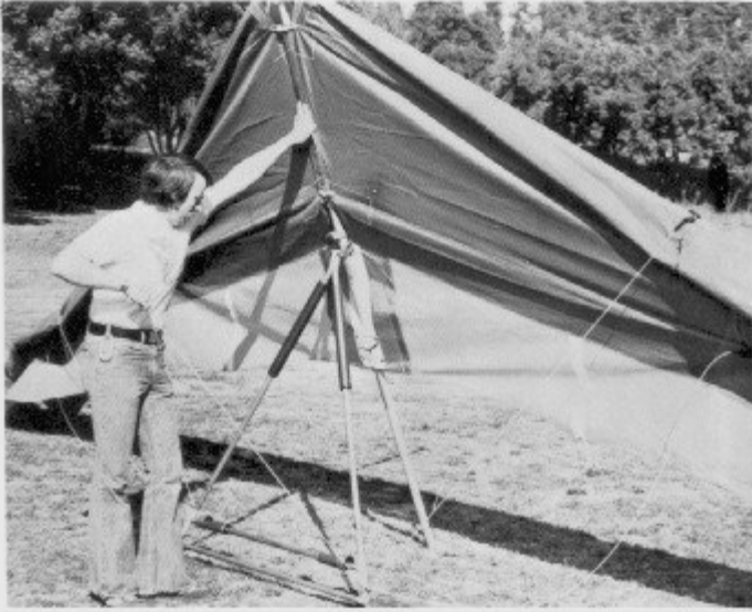
2. By lifting the nose and resting the wing back on its keel, you can swing the control bar forward.
