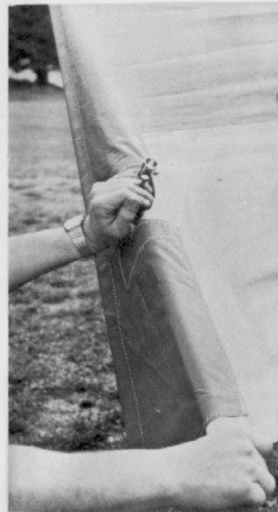
14. Insert the tip-rib into the rear spar bracket. Start by catching the edge with the bolt. At this point you can twist the tip-rib and it will align to the correct position.
