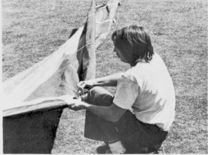
. With the keel spar against your knee, pull the nose-plate forward and insert the ball lock pin from above. Pull on the lower plate if necessary to get the BLP fully inserted. Make sure the spar do not slip off the rear spar in this operation.
