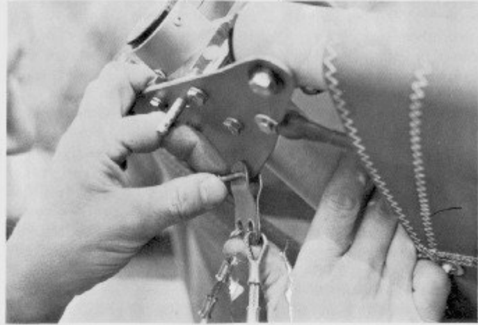
. Attach the nose-wire shackle to the nose plate with the clevis and safety ring. Note positioning of the hands to get enough slack.
