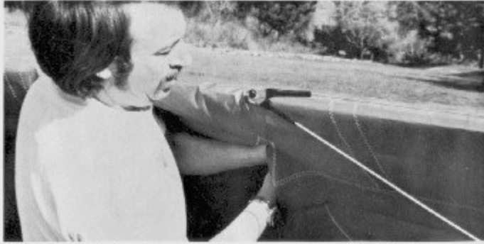
7. Assemble the four compression struts, starting with the two outside ones first. The struts are in two halves. Start by pulling back on the spring slide inside the forward half (attached to the leading edge). Just catch this insert inside the edge of the rear half of the compression strut , pull the compression strut straight , and then make sure the spring slide is slid all the way into the rear section . Be careful not to catch any fingers. Pull the zipper closed.
