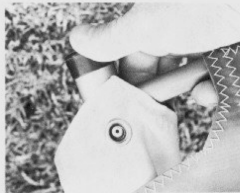
13. Pull the sail back and place the sail grommet over the peg at the end of the tip-rib, making sure the tip-rib and droop are aligned properly at the leading edge. (See #11)
