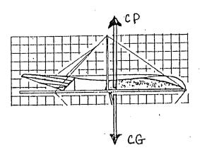
Trim speed is the speed at which a glider will fly placing the C.P. at the same point as the C.G. with no pilot input. This speed should be 2.5 mph above stall speed. A glider of good design and in good condition will produce bar pressure to return the glider to trim speed.
