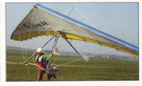
is due to the use of a mobile hanging integrated into the head of the frame: the wing is easy to pilot and turn, due to the absorption of shocks caused by turbulences on the roll axis.
